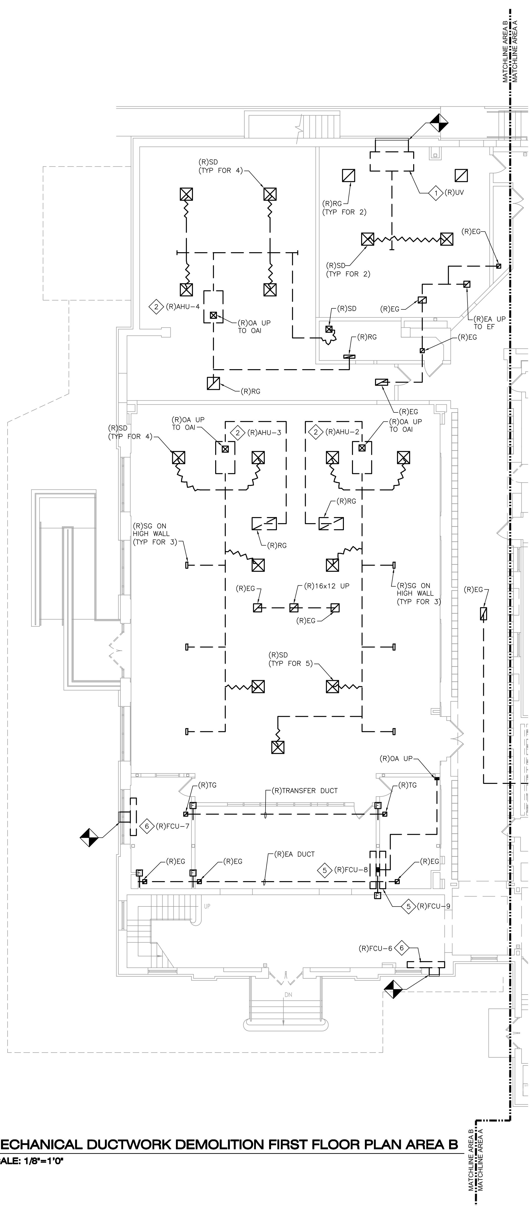
**1** MECHANICAL DUCTWORK DEMOLITION FIRST FLOOR PLAN AREA
